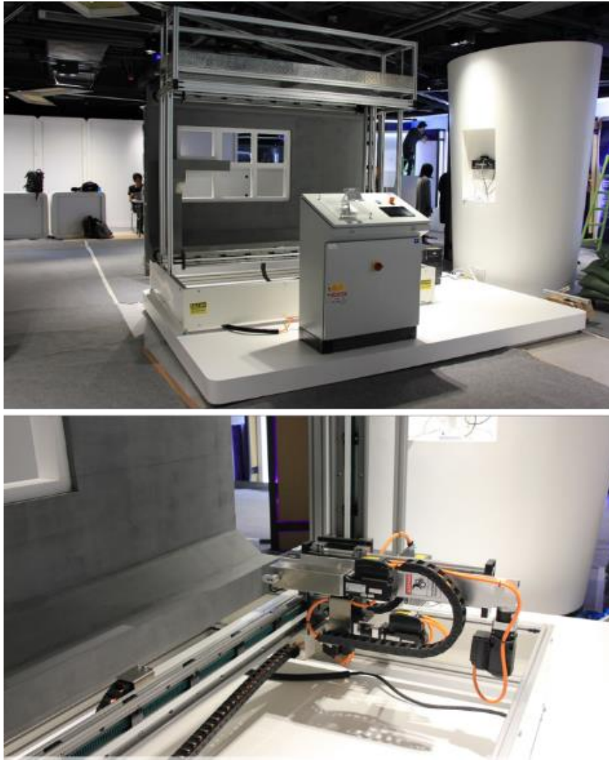
Figure 14 The semi-functional prototype of the multifunctional façade-processing robot displayed in the Construction Innovation and Technology Application Centre in Hong Kong (photo: R. Hu)
