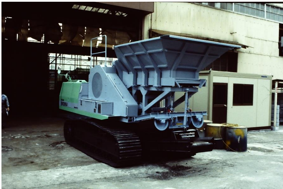
Figure 20 Concrete dismantling and recycling robot Garapagos (Photo: T. Bock)
