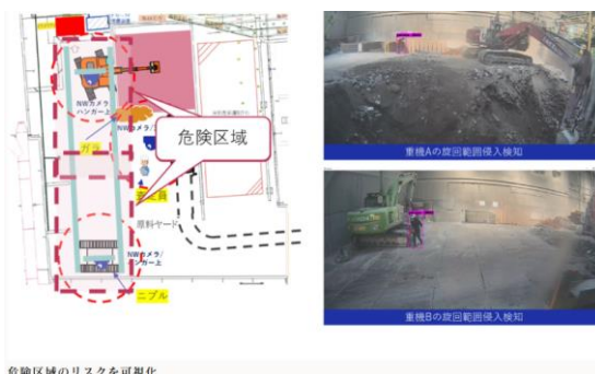
Figure 9 AI video analysis for hazard zone monitoring Figure 10 Remote operation setup for heavy machinery
