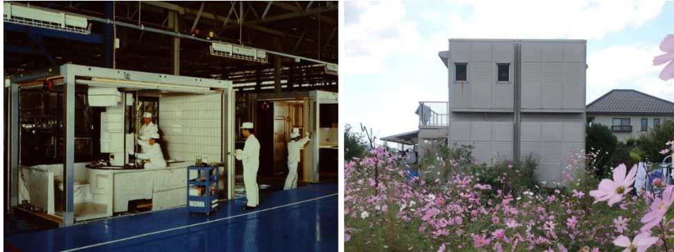
Figure 4 Stationary use of construction robots in the factory at Sekisui Heim and its legendary M1 model (photo: T. Bock)
