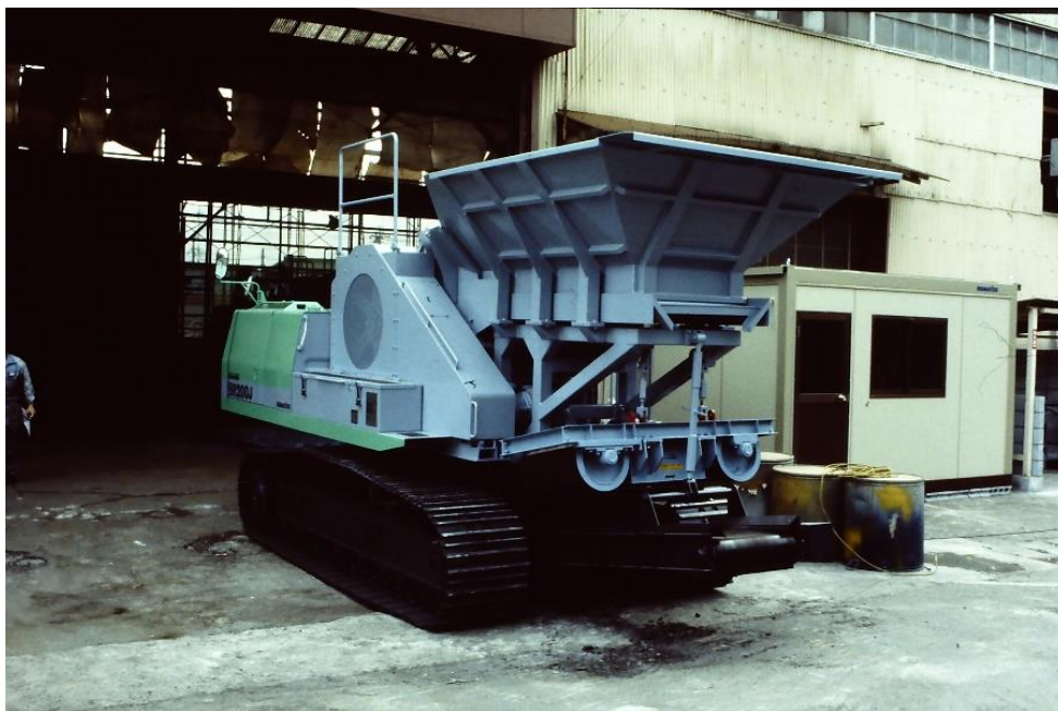
Figure 17 Concrete dismantling and recycling robot Garapagos (Photo: T. Bock)
