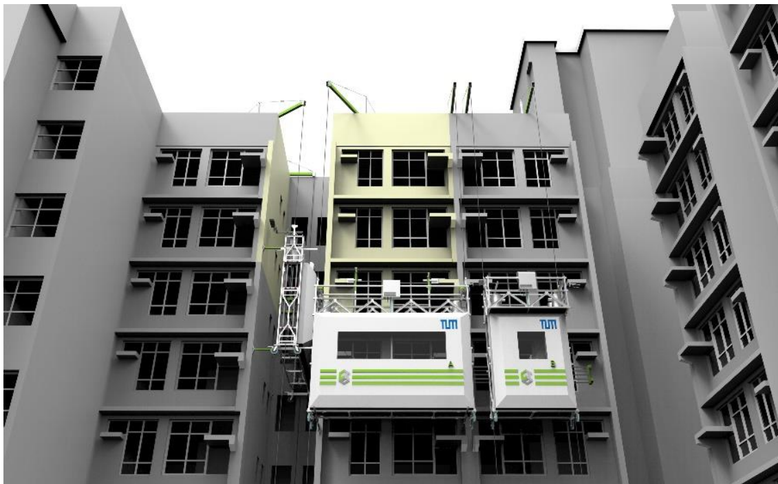
Figure 11 The multifunctional façade-processing robot showcasing the painting function on the façade of public housing buildings in Hong Kong (image: R. Hu)
