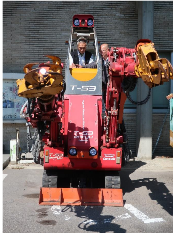
Figure 7 Maintenance robot Enryu T-53 developed by TMSUK Co. Ltd. (photo: T. Bock)
