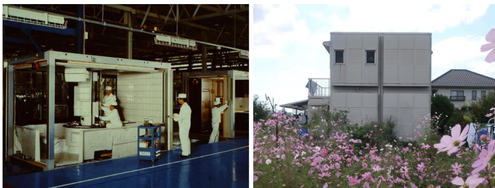
Figure 2 Stationary use of construction robots in the factory at Sekisui Heim and its legendary M1 model (photo: T. Bock)
